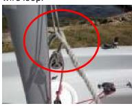
2.4 Tension the Jib until the Jib Luff (front edge) and the Shrouds are firm.
