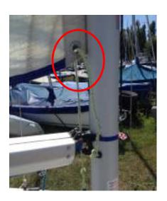
3.11 Secure the Knot at the end of the Cunningham into the slot beneath the gooseneck.
