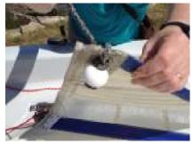
3.2 Feed the sail into the slot in the Mast.
