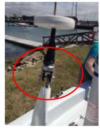
2.3 Hoist the Jib, until you can hook the jib tensioner through the loop in the wire Jib Halyard. NOTE: ensure that the rope tail is not trapped between the hook and the wire loop.
