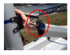
3.6 Insert the Slug (a bullet shaped object at the stern end of the sail) on the Clew of the Mainsail into the slot on the boom.
