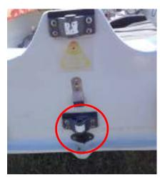
4.2 Place the Rudder into the Pintals, press it down until the spring clips. Then fit the ring through the hole at the bottom of the pintal to prevent the rudder from falling off.
