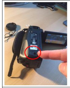
To Open the door to access the ports,
